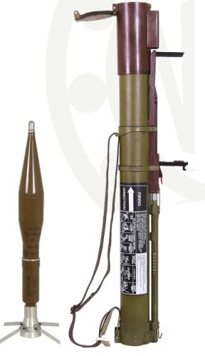
The RPG-22 rocket anti-tank grenade is a disposable individual weapon and is used against tanks, self-propelled guns and other armoured vehicles of the enemy, as well as against the enemy troops in the open, in bunkers, light field shelters and urban-type brick-wall fortifications.
