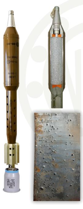
It is intended for use against enemy manpower located in the open, in trenches, field-type shelters or brick fortifications. The grenade is fitted with a warhead containing prefabricated fragments and a more powerful explosive that almost doubles its combat power.
