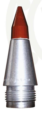
The V-5K fuze is intended for use on the S-5K, S-5KO, S-5MO and UAR-57TB unguided aicraft rockets. It serves to ensure their safety during handling and firing and to detonate the rocket's warhead on impact with a target. The fuze is nose, impact with instantaneous and inertial action, non-boresafe type.
